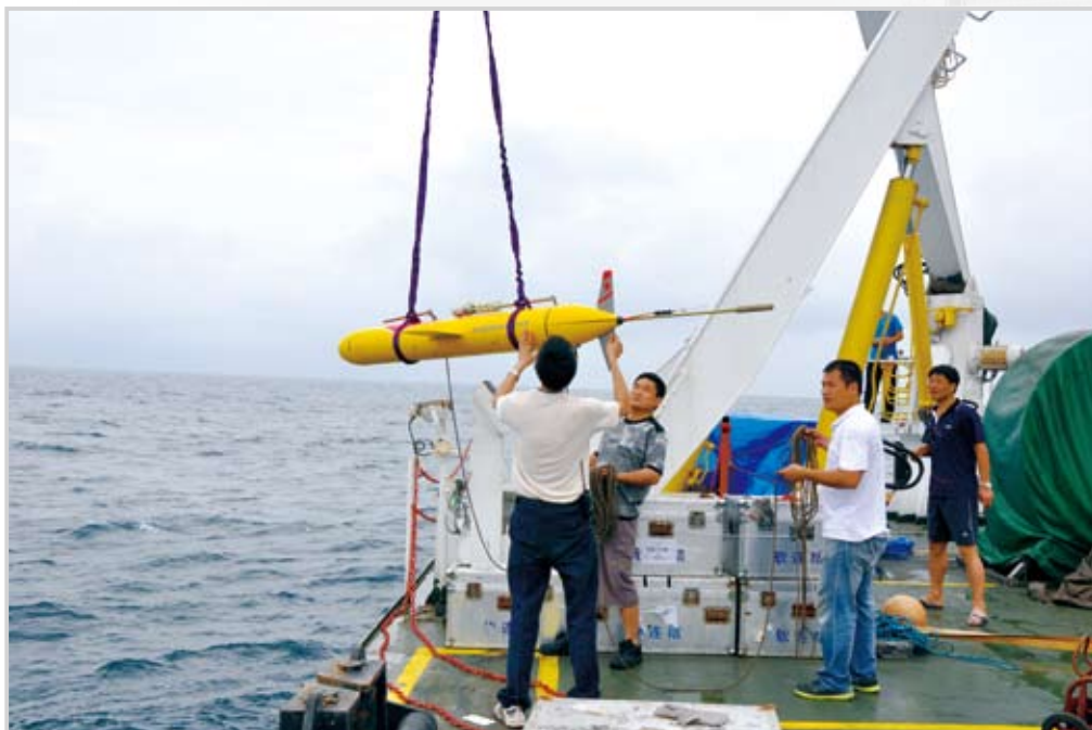
● “实验1”科考船在海上做水下滑翔机试验
